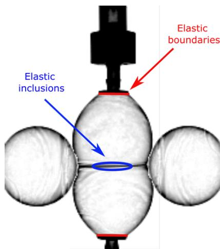
Figure 1: Schematic view of two interacting bubbles in complex environments: many bubbles; flexible boundaries; elastic insertions.
